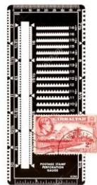
Instanta gauge provides sliding scale of perf measurements with lines printed on clear, thin plastic
